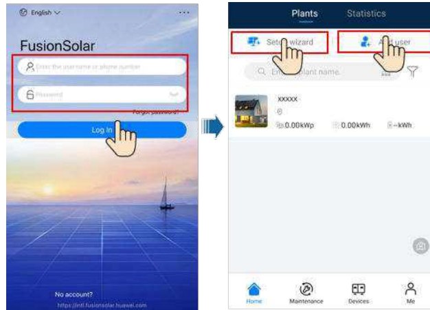
Figure 7-5 Creating a PV plant and a user
