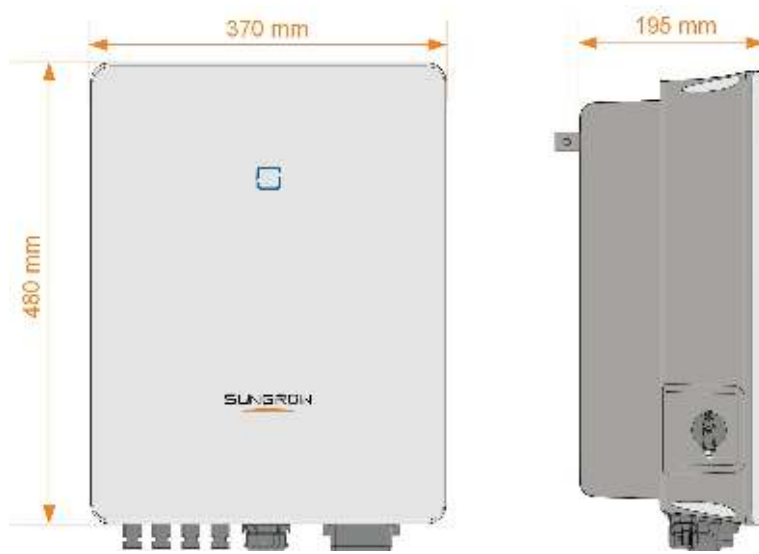
Figure 2-3 Dimensions of the Inverter(in mm)
