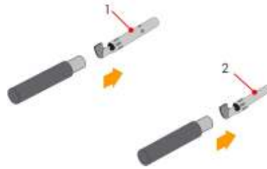
1: Positive crimp contact
