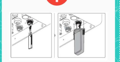
The Wi-Fi dongle is located on the rightside underneath the inverter with a grey cover.
