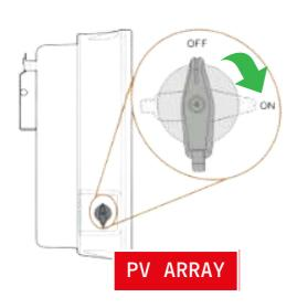
Turn on the PV Array DC Isolator
